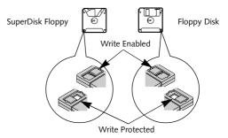
Figure 4-5 Floppy Disk Write Protect
